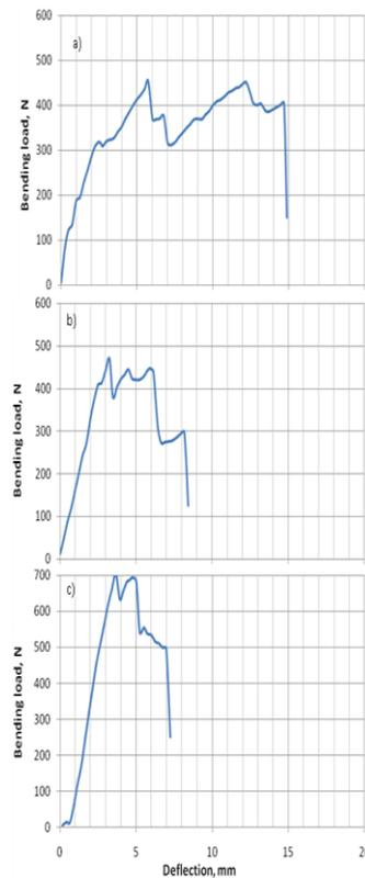
Fig 2. Bending load Vs deflection of a) sinusoidal b) Square and c) triangle core corrugated sandwich with 0.75 mm thick corrugation under three point bending.
