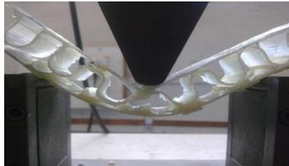
*Three point bending test of a specimen using UTM*
